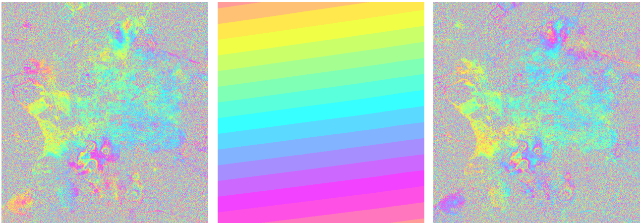
Figure 4: Left: Original interferogram, Middle: Linear phase trend, Right: Interferogram after remove of the linear trend
